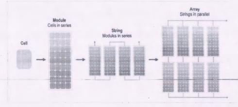
Figure 2: Depicts the Solar Cell to Solar Array.
